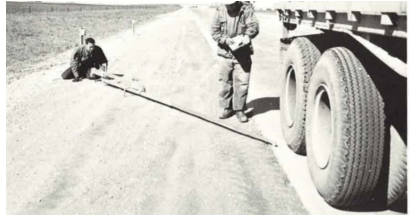
Figure 37. Measuring static rebound deflection with the Benkelman beam.
